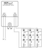
Hot plug-in or secondary switching is not permitted.
